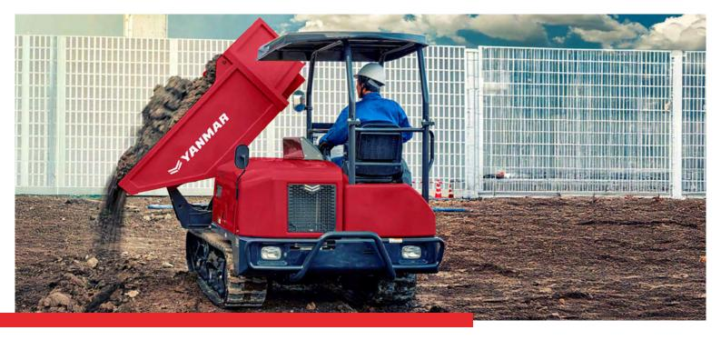
Lynch operates a modern and reliable fleet of Swivel Tip Tracked Dumpers, offering **180° rotation** allowing for loads to be tipped in any direction. This increases the efficiency of the machine and the productivity of the operator.
